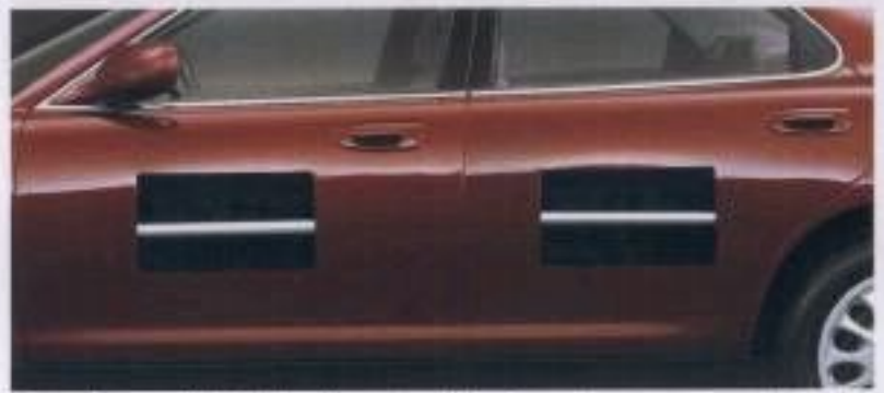
Every door panel is fitted with an impact bar for extra passenger protection in the event of a side impact. And the extra-strong door latches minimize the possible danger of passengers being thrown out.
