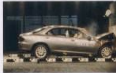
The ELINOS 500 meets the impact resistance requirements of the United States, which has some of the world’s most stringent safety standards. Tests include 50kph head-on and rear-end collisions. Door latches, too, have added strength.
